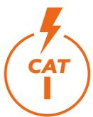
Measurements on circuits not directly connected to the distribution network
